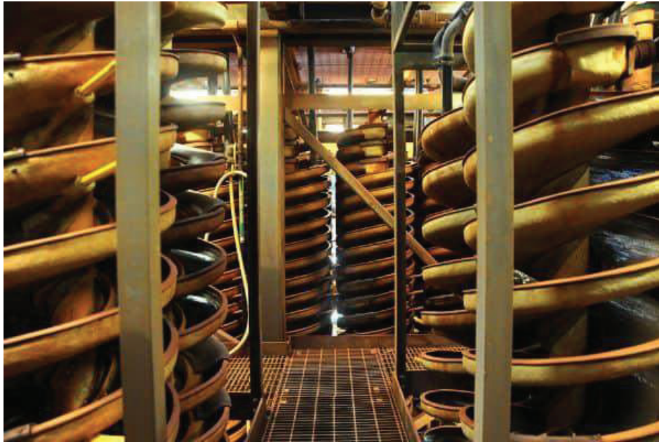
Fig. A – Parallel Spiral Gravity Separation Modules - The ore is washed through a series of spiral separators to separate the heavy mineral content from the lighter quartz and clay impurities.
